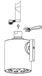
Apply pipe tape on the threads of shower arm (which is not included in this product package). Tighten the shower head to shower arm with wrench.
